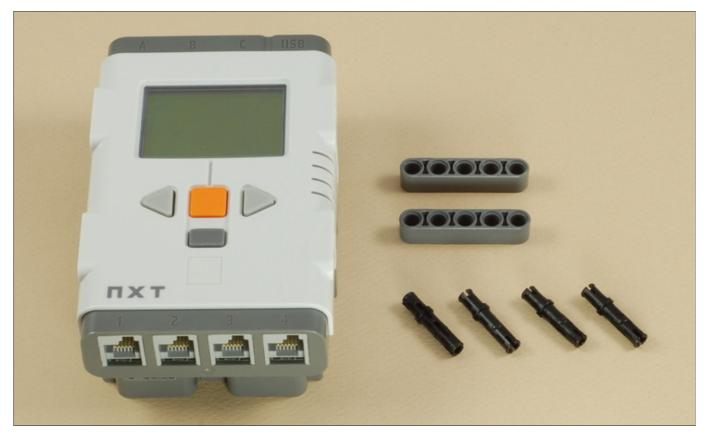
**Note:** You can use the NXT with either AA batteries or the NXT Rechargeable Battery Pack.
